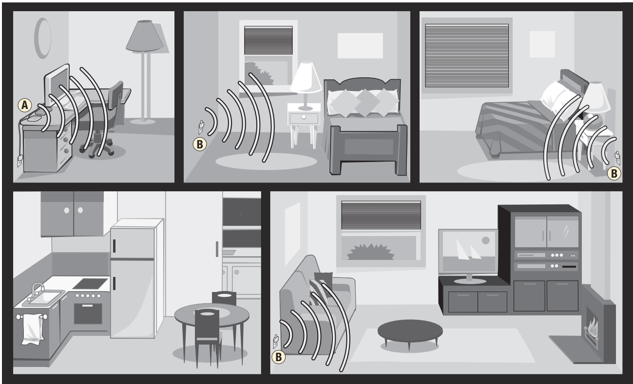
This illustration shows an example set-up of the Platinum App Bridge (A) and Platinum Repeaters (B).
